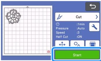
**7** If the backing of the template sheet is cut, adjust the Cut Pressure(Half Cut) to lower it.
